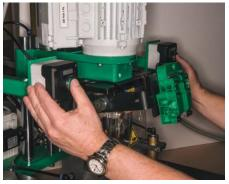
**Pneumatic controls** Two-hand start button controls for safe drilling and insertion functions.
